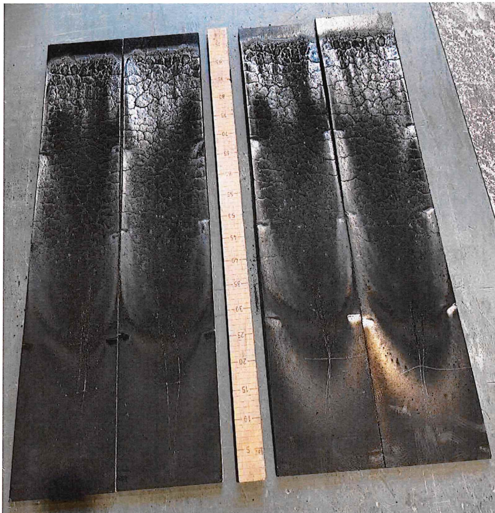
Fig. 4: Illustration of the specimens of Brandschacht test 1.
